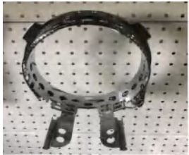
Cap rings 8 sets snap into cap station for embroidery preparation
