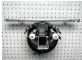
270° cap driver 3 sets snaps into bracket holder for the machine hoops
