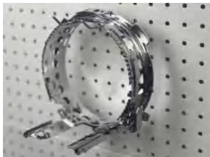
Cap rings 2 sets snap into cap station for embroidery preparation
